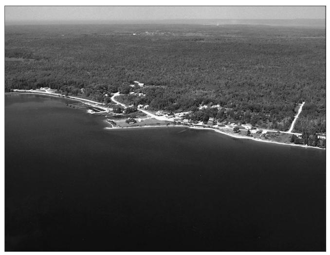
146 The L-shaped Public **wharf** at Meldrum Bay is 2.4 m high. The outer face is 27 m long with depths of 5.2 m. The north face has depths of 1.8 to 3.7 m and the south face 0.9 m. There is a building on the outer end of the wharf.
