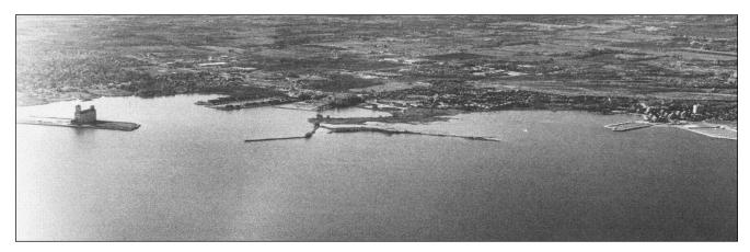
outer end. On the SE side of the harbour there is a rubble **breakwater** with a concrete pier extension and a north arm.
