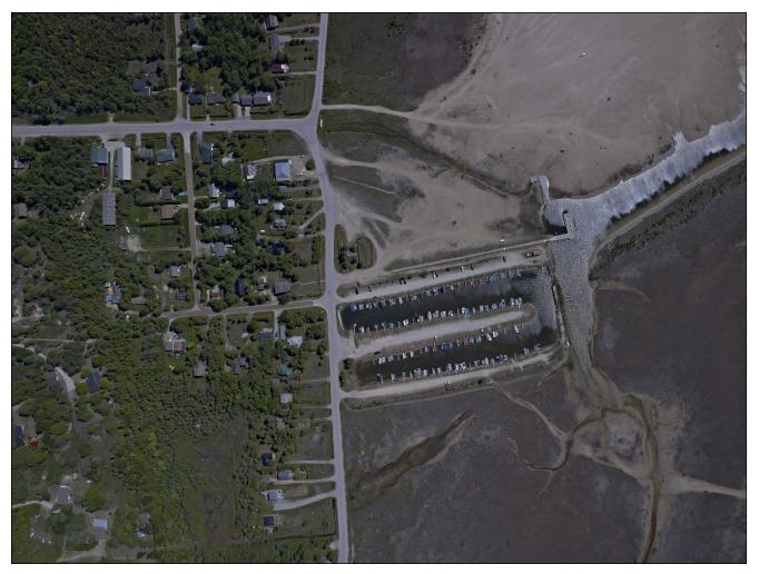
241 The **Public wharf** at Oliphant is at the outer end of a **causeway**. The wharf is L-shaped with an outer face 84 feet (26 m) long and has depths of 4 to 8 feet (1.1 to 2.3 m) (1994). Commercial fishing boats use the wharf.
