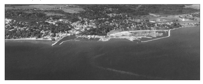
The angled east pier is connected to a rubble breakwater which forms the south wall of a sheltered basin used by fishing vessels. The harbour extends 0.5 mile up Lynn River and into **Black Creek**. A marina 0.3 mile east of the main harbour entrance is protected by a rubble breakwater.
