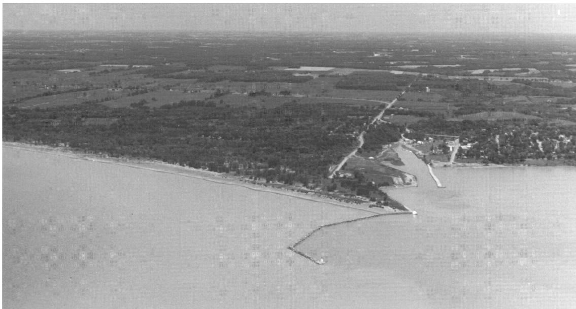
The east pier extends 1,000 feet (305 m) from the shore. An area of landfill on the west side of the harbour entrance reaches 0.2 mile farther south and is fronted by a breakwater wall. A boulder breakwater at the south end of the breakwater wall extends another 0.25 mile to the SSW and has an elevation of 10 feet (3 m).
