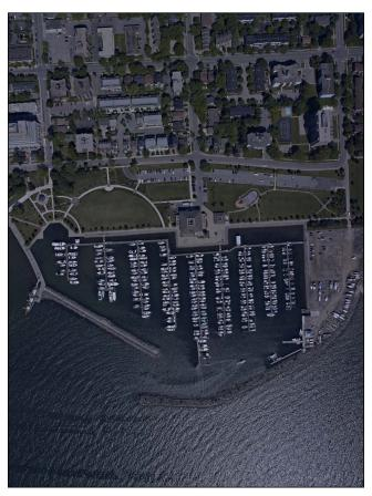
Inside the harbour entrance, the channel follows along the north pier. Bronte Harbour is subject to **silting**. Depths of 6 feet (1.8 m) were found in the harbour channel in 1994. A highway **bridge** across Bronte Creek at the upper end of the inner harbour has a vertical clearance of 20 feet (6.1 m).
