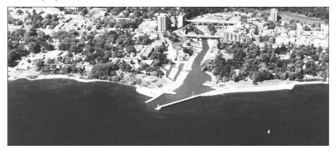
(23 ft) in 1995; an inner berth on the SW side, 91 m (300 ft) long, had a least depth of 6.1 m (20 ft). In addition to facilities for loading and discharging fuels, ballast water can be discharged ashore.
