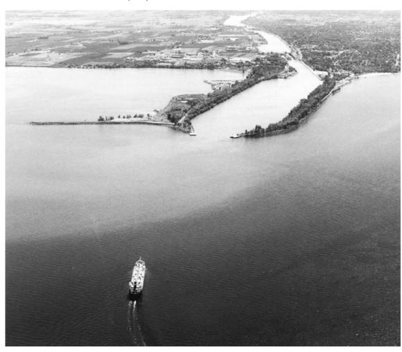
The harbour is entered between two concrete piers, 182 m (597 ft) long, including the pier heads. The centre line of the entrance bears due south, as does that of the harbour for a distance of 1.2 miles from the entrance. At this point the centre line deflects 15° to the east to align with Lock 1, which lies 0.4 mile farther south.
