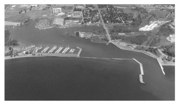
its SE corner between two concrete piers which extend out from shore. The west entrance pier has an elevation of 2.4 m (8 ft); a rubble breakwater extends 91 m (300 ft) southwards from its outer end. The east pier has an elevation of 2 m (7 ft).
