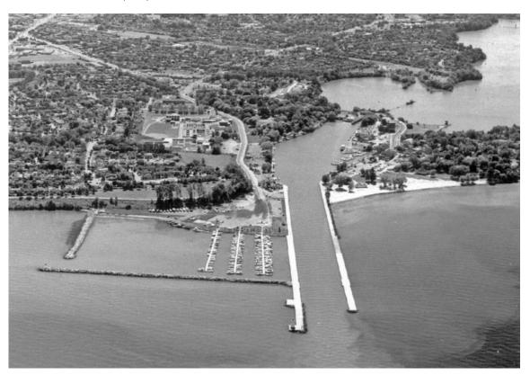
(1,312 ft) wide at the *Beacon Harbourside Inn*. The breakwaters, which protect a marina basin, have an elevation of 3 to 4 m (10 to 13 ft). An opening near the NW corner is marked by a starboard hand **daybeacon** on the south entrance wall and Jordan Harbour light on the north breakwall.
