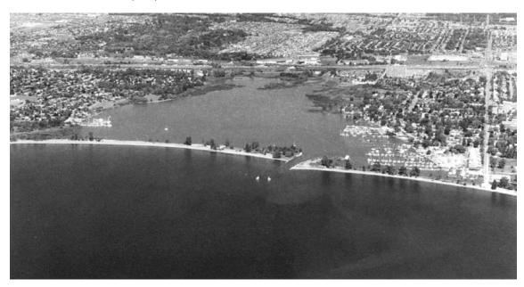
a narrow sand bar named **Fairport Beach**. The *Pickering Generating Station*, to the east, makes a good landmark for locating the bay. The bay is entered between two parallel breakwaters,  $30 \, \text{m} \, (100 \, \text{ft})$  apart, extending  $122 \, \text{m} \, (400 \, \text{ft})$  into the lake. A sandy beach extends westward from the entrance.
