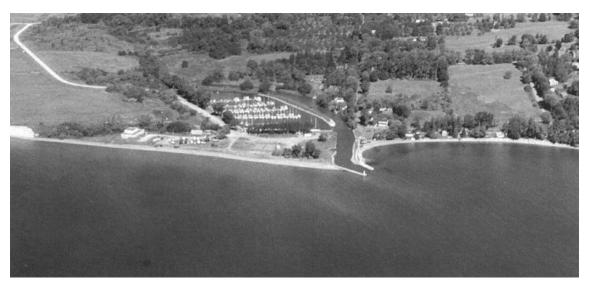
elevation 6 feet (1.8 m). The west breakwall has a total length of 302 feet (92 m), with the outer 180 feet (55 m) being a sheet piling and concrete pier, elevation 6 feet (1.8 m). Due to the configuration of the shore the west entrance pier extends farther into the lake than the east pier.
