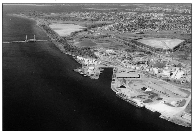
berths. The north berth has a total length of 622 m, with a deck elevation of 4 to 4.3 m. The southern berth has a length of 274 m, with a deck elevation of 4 m. On the north side of the basin is a warehouse, 122 by 76 m. On the south side is another warehouse, 61 by 30 m.
