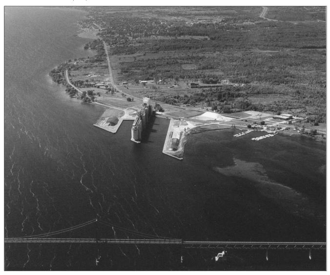
106 **Ogdensburg-Prescott International Bridge**, a high-level suspension **bridge** with a vertical clearance of 40 m, spans the river between **Johnstown** and the U.S. shore 2 miles NE of Ogdensburg. The main piers, elevation 84 m, are 350 m apart. White **lights** are shown from the main towers on each side of the channel; a green **light** shown from each side of the main span indicates the centre of the channel. The main towers have air obstruction **lights**.
