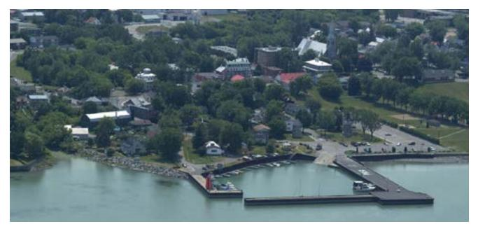
with an outer end 25 m in length with a depth of 1.8 m alongside; there is a **ramp**. The lower section of the wharf may be submerged during runoff periods.
