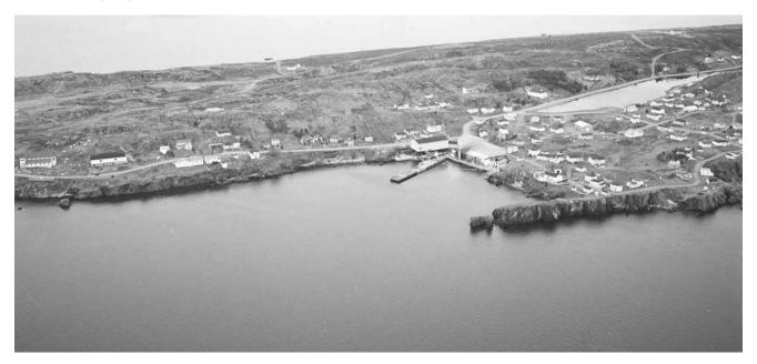
near the head of the harbour. The east **wharf** extends 107 m (351 ft) from the shore with a bent outer end 17 m (56 ft) long. Depths of 1.3 to 2 m (4 to 7 ft) exist alongside the wharf. A **light**, privately maintained, is located at the outer end of the wharf. Several floating wharves are moored on the south side of the wharf.
