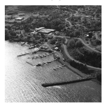
On the SW side of Dark Hole is the *Clarenville Marina*. The marina, which can accommodate 70 boats, consists of floating wharves which are equipped with 15 and 30 amp electric power; fresh water is available. Protection is afforded by a stone breakwater which extends 105 m (344 ft) SE from the shore, close north of the marina.
