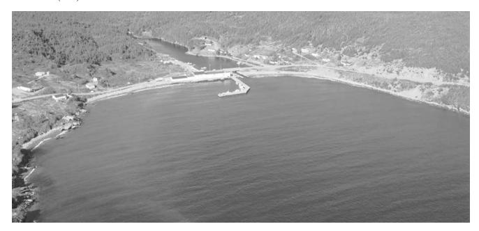
(266 ft) to a depth of 3.3 m (11 ft) alongside an outer end 43 m (141 ft) long. A **light** (508.5) is shown from a mast on the outer end of the wharf. A canal, with a depth of 0.9 m (3 ft) in an entrance 9 m (30 ft) wide, leads to a small basin close NW of the wharf. There is a clearance of 2.7 m (9 ft) under the bridge spanning the canal. A floating wharf and a boat
