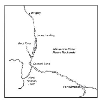
Between Kilometres 534.3 and 566.5 the current is swift and seething but the navigation channel is well marked by beacon ranges. The settlement of Wrigley lies on the east bank at Kilometre 572.9.
