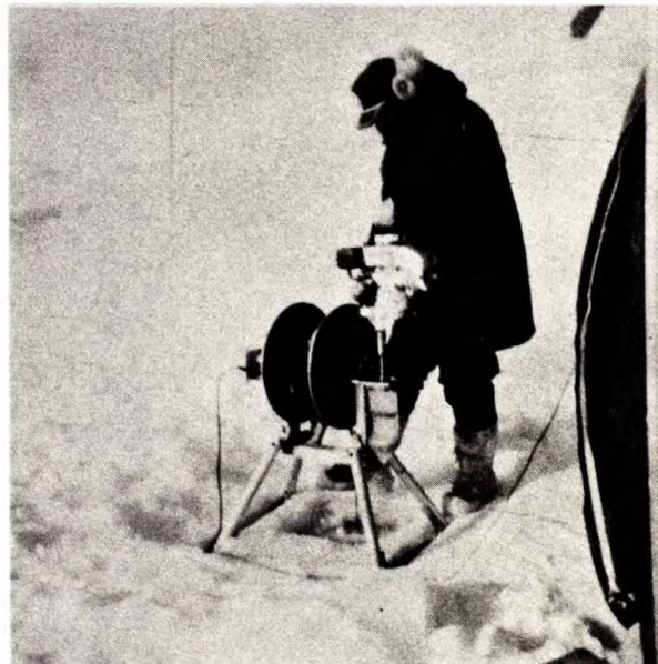
Plate 4. The first prototype winch: Jiffy auger power head employed to haul up CTD.
