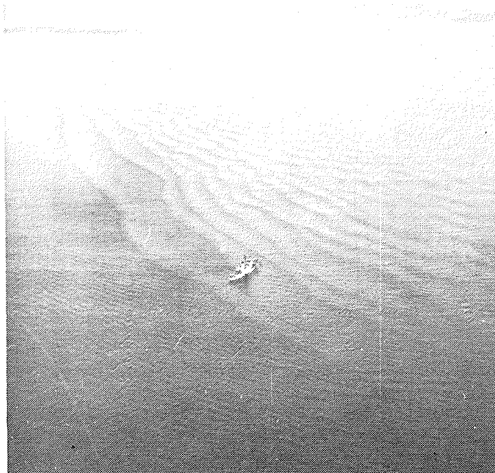
An airphoto of the research vessel "Endeavour" making measurements of an internal wave packet in Georgia Strait. Airborne and satellite images taken at the same time will be used to test theories of the radar imagery process and to evaluate the radar for future oceanographic programs.
