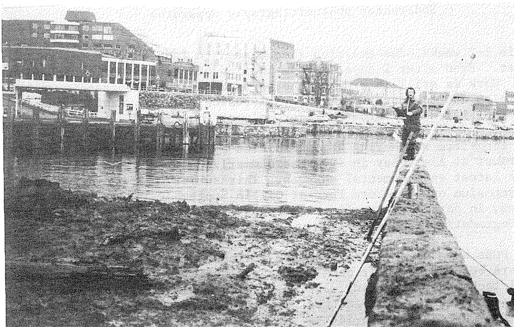
Sampling dredge spoils in Victoria's Inner Harbour for Determination of trace metals, hydrocarbons and other environmental contaminants
