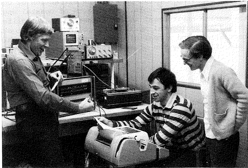
J. Love, D. Smith and T. Curran with Aanderaa tape translation system. Data, recorded in coded form in submerged instruments, is read from recovered tapes and translated into computer compatible format for processing.
