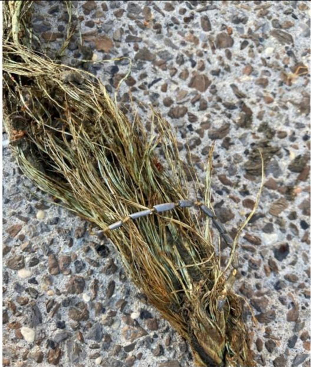
E04-21 image – Sink line showing the beaded lead yarn.
