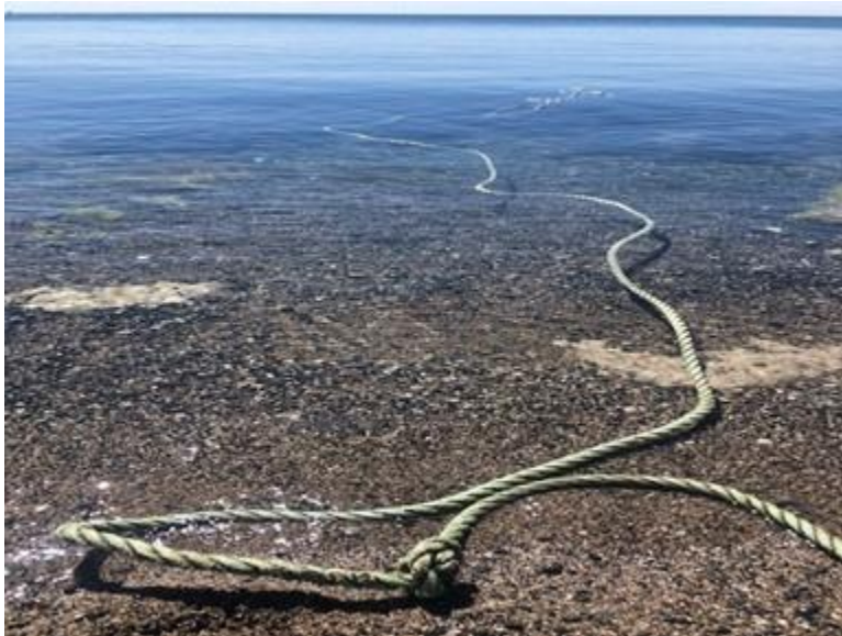
Figure 4. Same rope as in Figure 3 showing its positive buoyancy. The irregularity in the line is a cinched loop (Photo credit: E. Trippel).
