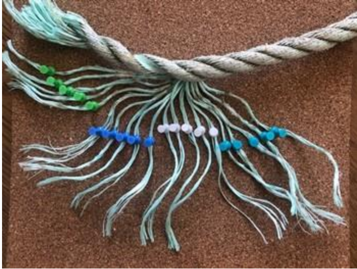
Figure 5. 5/8 inch diameter float rope removed on May 12, 2021 showing its construction composed of 20 twisted bundles in each of the three strands. (Photo credit: E. Trippel).
