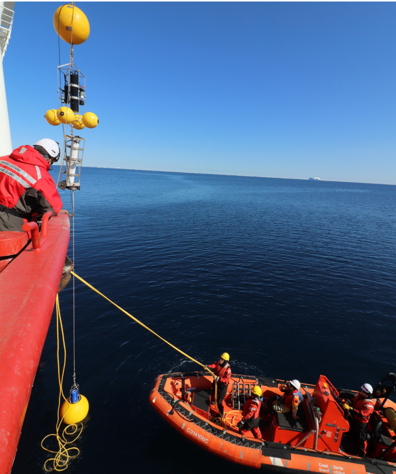
Deployment of a mooring from CCGS Amundsen with support from the vessels zodiac. Photo credit: Megan Lee (DFO).
