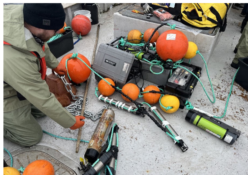
DFO Science and local harvester deploying sound-trap for acoustic monitoring. Photo credit: Lee Sheppard.
