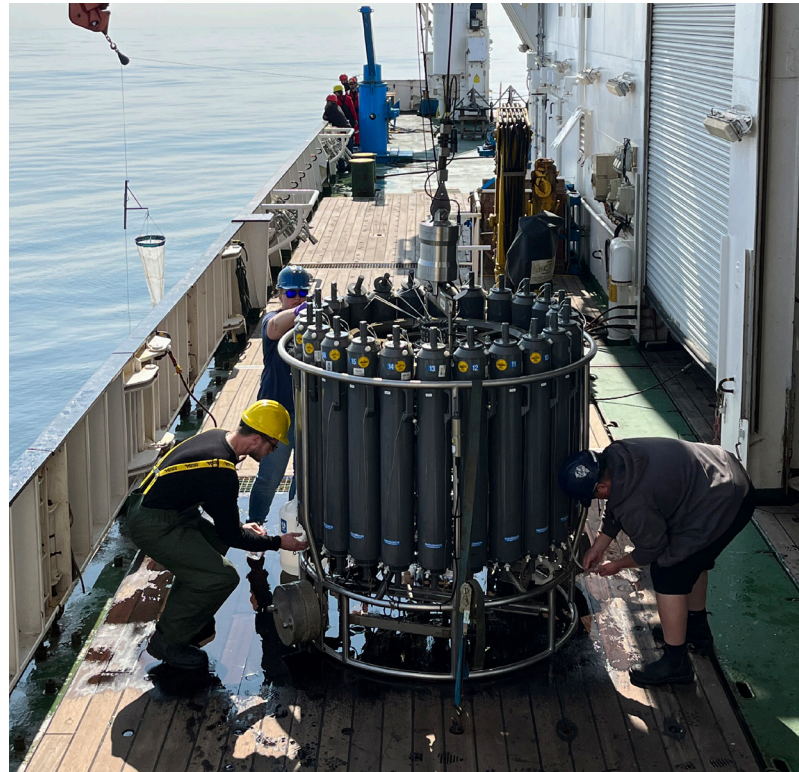
A CTD rosette, used by the Atlantic Zone Monitoring Program. Photo credit: DFO.
