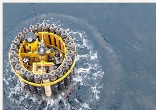
CTD-Rosette (conductivity, temperature, depth) Sampling instruments being deployed. © Fisheries and Oceans Canada
