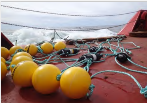
Acoustic telemetry receivers on mooring lines. © Susan Heaslip (Fisheries and Oceans Canada)
