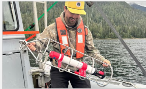
Conductivity, temperature and depth (CTD) sensor. © Amy Elvidge (Fisheries and Oceans Canada)
