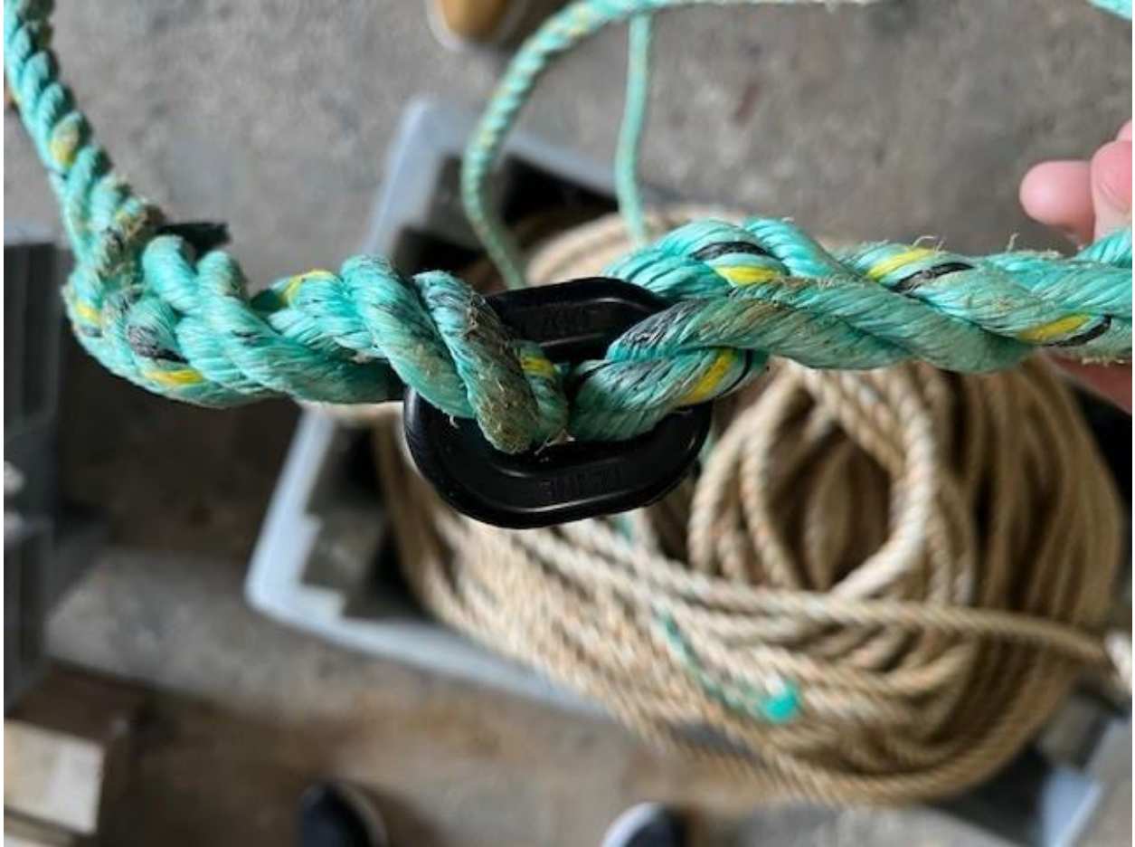
Fig. 3. An example of a Maine Mold weak link inserted in a buoy line with lazy man splices using several tucks (Photo credit: E. Trippel).
