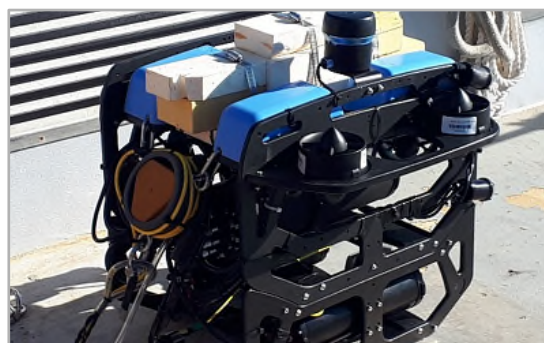
"Blue ROV2" used to survey anchorage sites. © Cathryn Murray (Fisheries and Oceans Canada)
