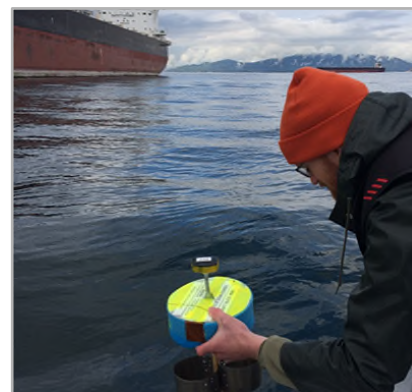
Deployment of a current tracking drifter. © Roy Hourston (Fisheries and Oceans Canada)
