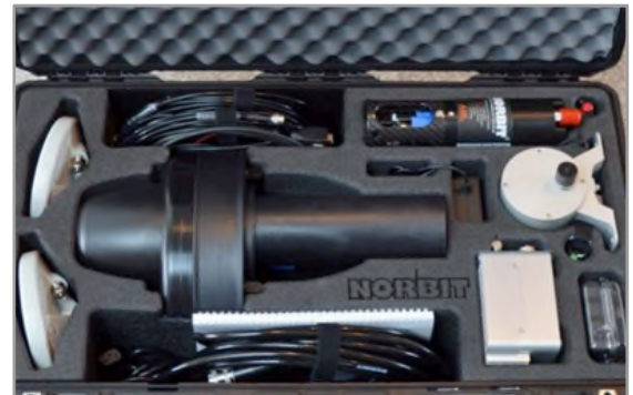
Portable multibeam echo sounder (Norbit) equipment.
