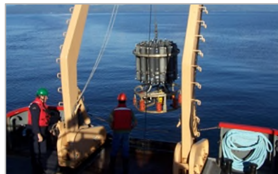
Deployment of a rosette, a deep water sampling apparatus.
