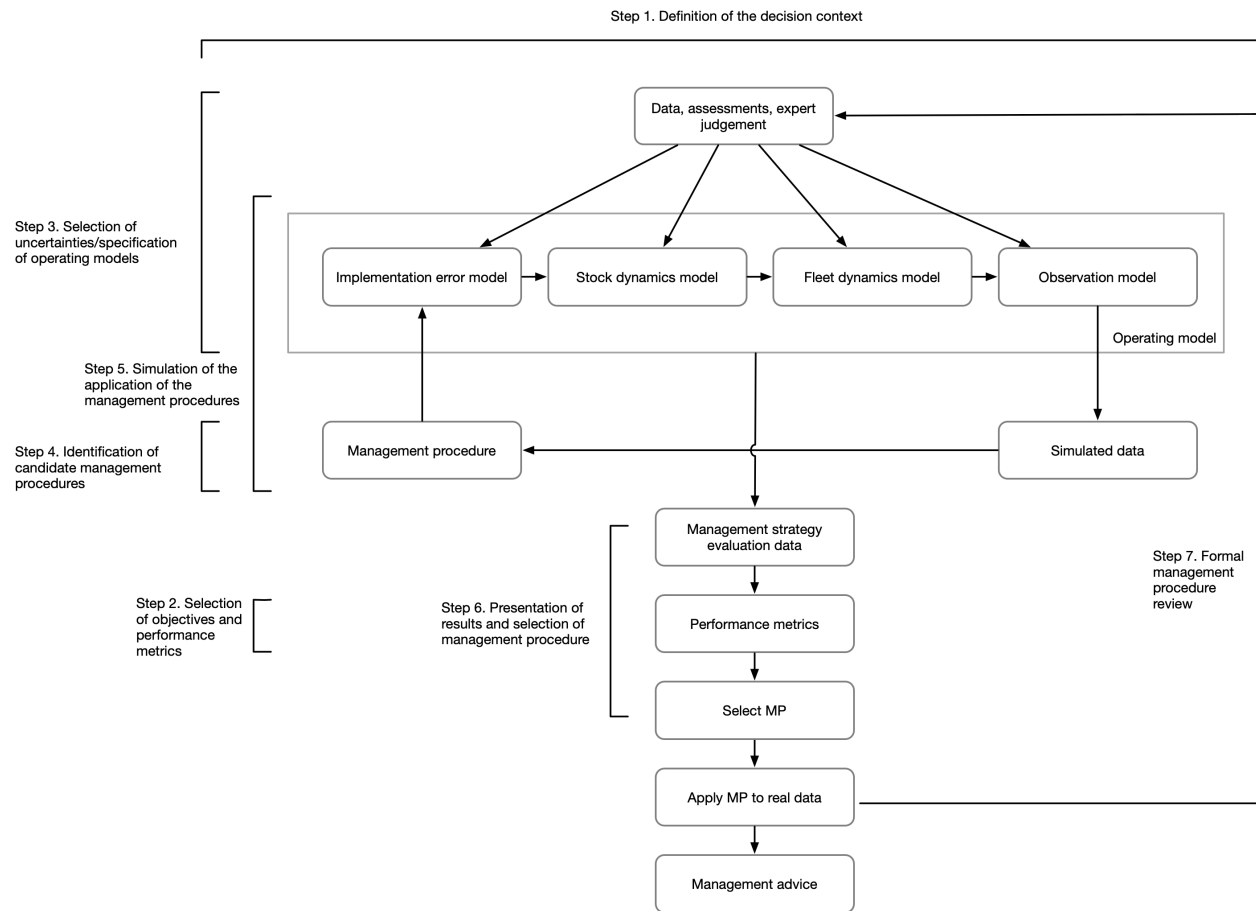
Figure 4. The steps of the MSE process following Punt et al. (2016) as implemented in openMSE, copied from Anderson et al. (2021) and adapted from Carruthers and Hordyk (2018a). This figure expands on Figure 3.
