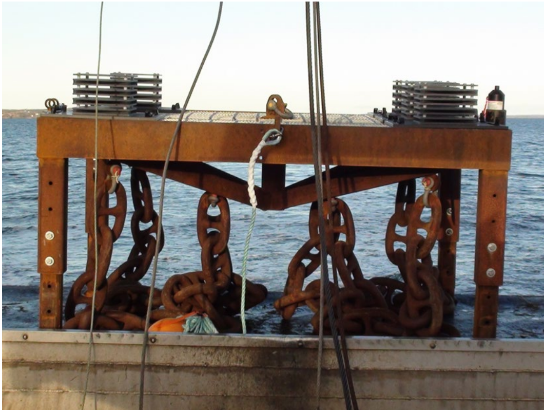
Figure 10. A permanent mooring located at the Scatarie Bank Experiential Research Site within St. Anns Bank MPA. The platform hosts several Autonomous Reef Monitoring Structures (ARMS), and instruments to record temperature and salinity over time.
