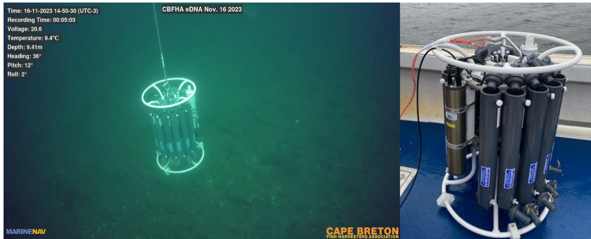
Figure 14. Deployment (left) of a water sampler rosette by the CBFHA used for eDNA sampling. The rosette (right) contains Niskin bottles to collect water samples at specified depths, and a CTD to record temperature and conductivity profiles of the water column.
