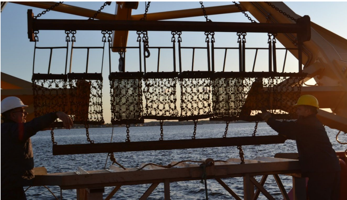
Figure 6. Research survey gear composed of a toothed 8-gang scallop drag (82.6 mm rings) with two of the drags lined (18 mm mesh) used in the 2019 and 2023 scallop surveys in the southern Gulf of St. Lawrence.
