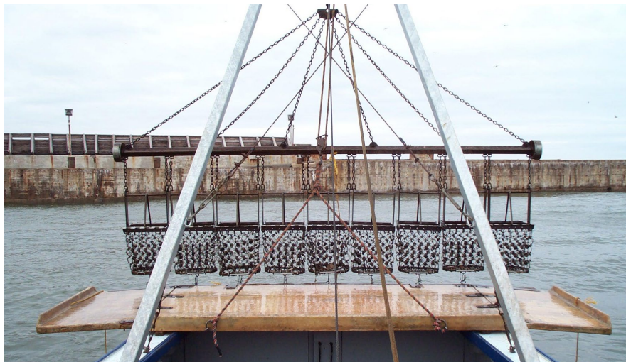
Figure 2. Nine gang Digby-type dredge commonly used to fish sea scallops in the Gulf Region.
