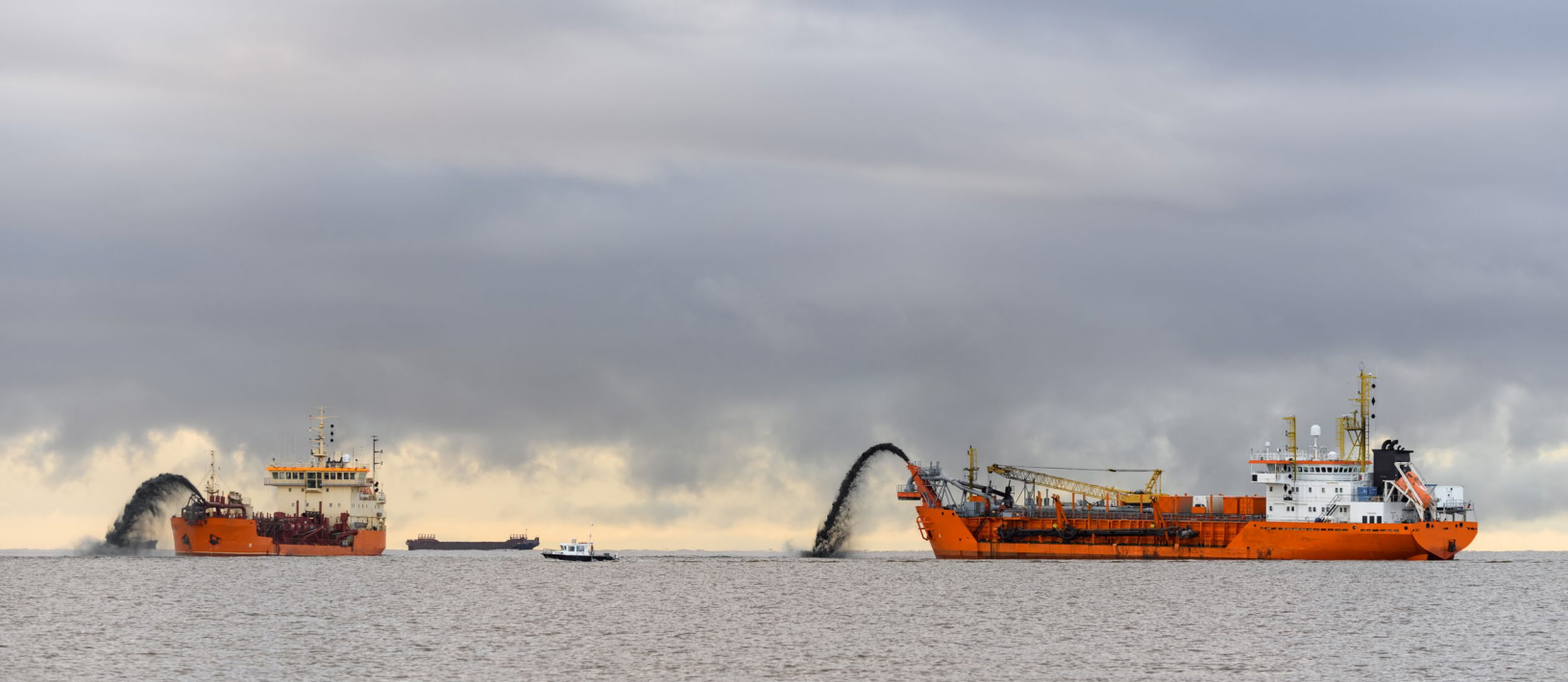
Two suction hopper vessels engaged in dredging. Credit: Alexey Seafarer.
