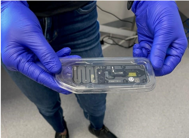
Image 1: The SpotON Flow Cell unit used for MinION Mk1B nanopore-sequencing.
