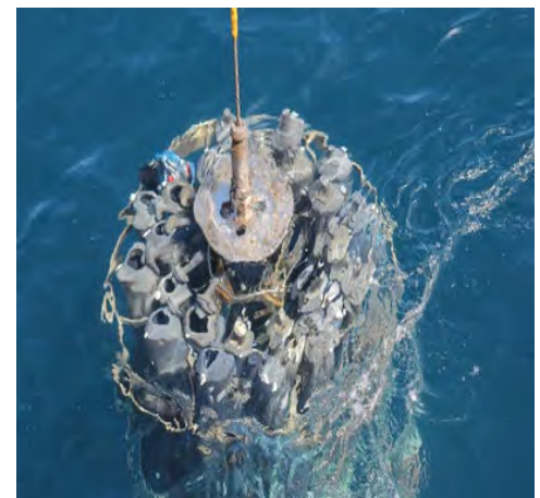
Image 2: Deployment of a rosette, a deep water sampling apparatus. Credit: Fisheries and Oceans Canada
