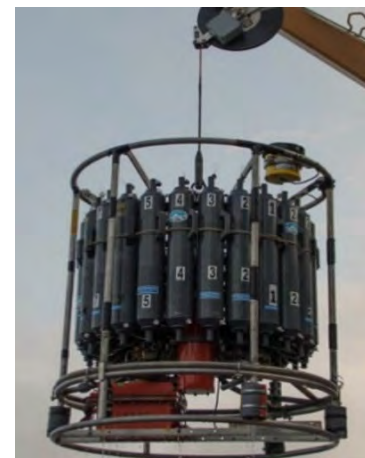
Image 2: Deployment of a rosette, a deep water sampling apparatus. Credit: Fisheries and Oceans Canada
