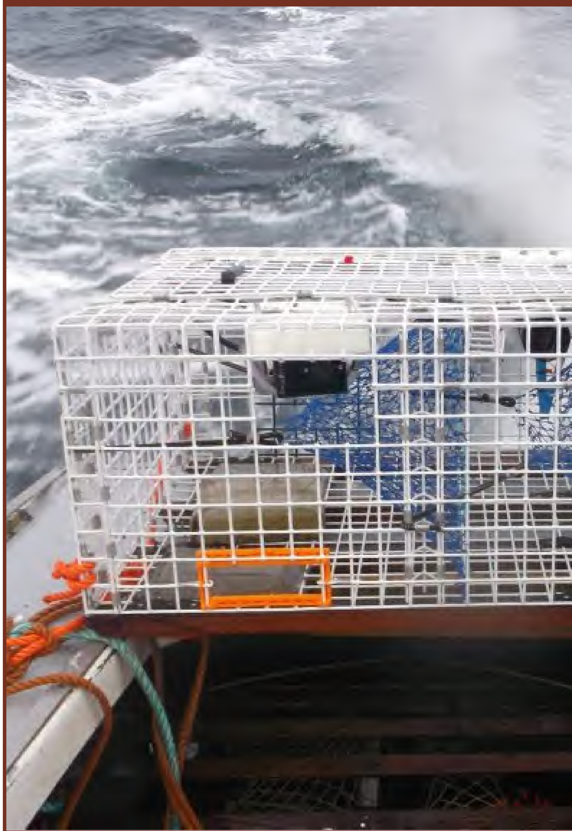
A BRUV system ready for deployment in St. Anns Bank Credit: Cape Breton Fish Harvesters Association
