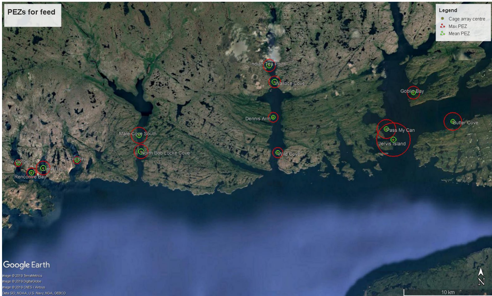
Figure 15. Google Earth image showing the location and size of mean (green) and maximum (red) PEZs associated with the release of waste fish feed pellets from proposed sites.
