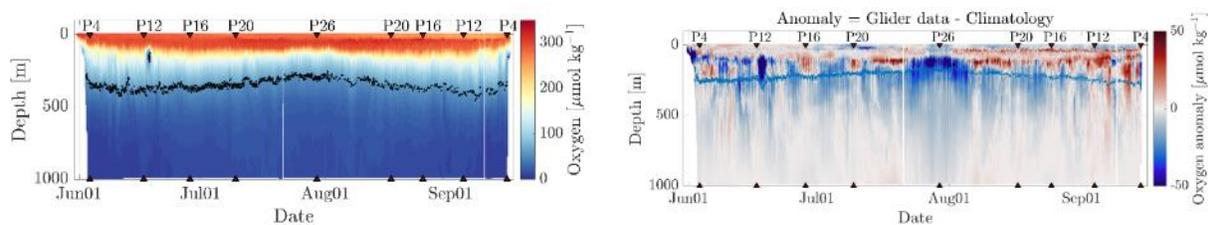
Figure 13-4. Transect of ocean glider oxygen concentration along Line P from P4 to OSP between May and September 2022 as a function of depth and time (left). The black dots show the 60 μmol/kg surface, indicating the hypoxic boundary and the approximate top of the OMZ. Oxygen anomaly along the same transect (right). The blue dots show the location of the 1026.7 kg/m<sup>3</sup> isopycnal.
