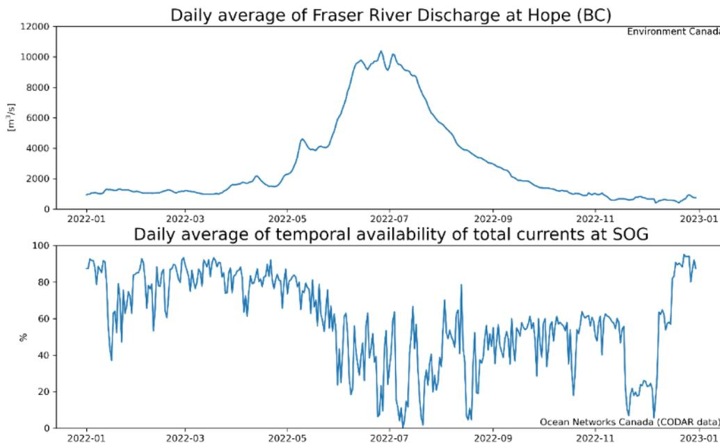
Figure 38-6. The Fraser River discharge [ $m^3/s$ ] at Hope (top) and the percent good (# of cells returning good daily data) CODAR data for the Strait of Georgia. The slightly late freshet, resulted in a drop in CODAR data coverage from late June through into August.
