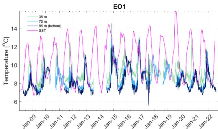
Figure 12-2. Temperature time series at E01 mooring for different depths: the surface (satellite SST), 35 m, 75 m, and 95 m.
