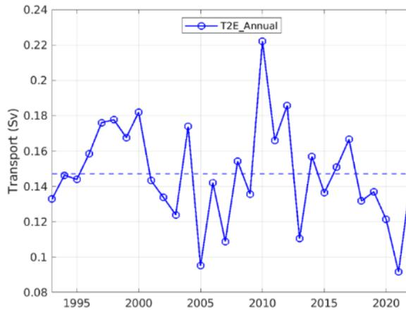
Figure 14-3. Annual-mean water transport (positive poleward) associated with the Vancouver Island Coastal Current. The dashed line is the mean transport averaged over 1993-2022.  $1 \text{ Sv} = 10^6 \text{ m}^3/\text{s}$ .
