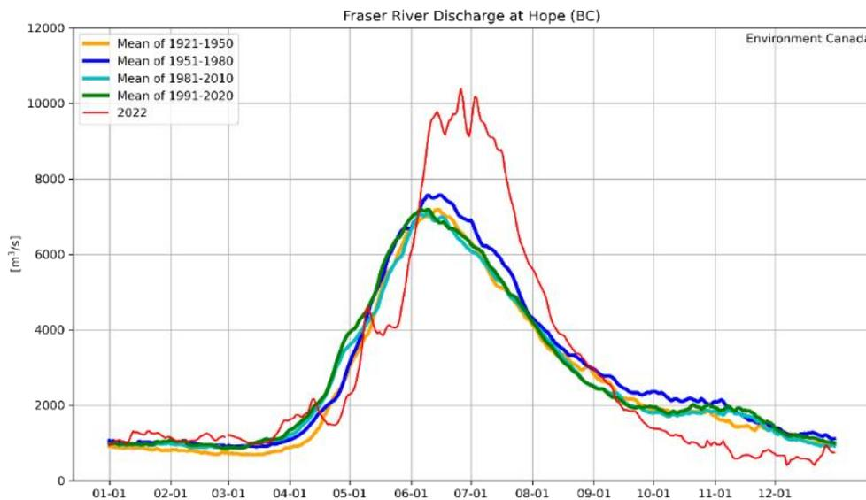
Figure 38-4. Fraser River discharge ( $m^3/s$ ) at Hope as reported by Environment Canada. Shown are three 30 year climate averages and the discharge curve for 2022 (red). A three week cooling period in May 2022 delayed the freshet, which then peaked in late June (rather than early June) at relatively high levels ( $10,000 m^3/s$ ).
