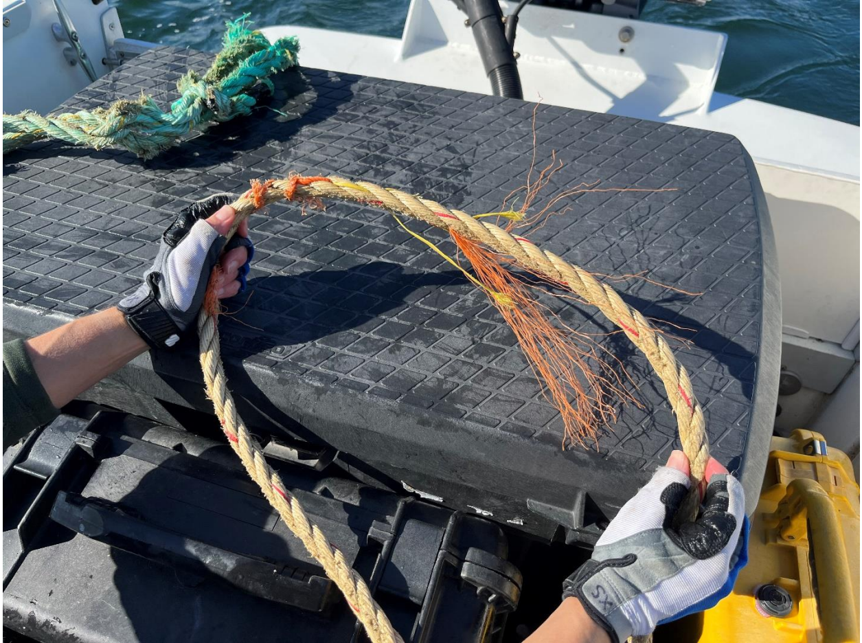
Fig. 2. Orange and yellow twines interlaced along the same section of rope. Photo credit: Georgia Department of Natural Resources
