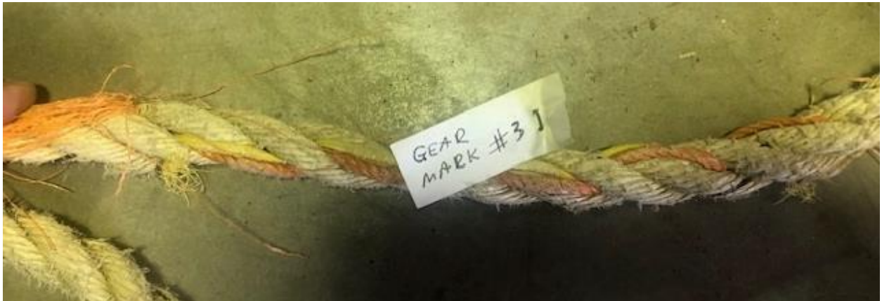
Fig. 8. Third occurrence of orange and yellow twines interlaced along the same section of rope.
