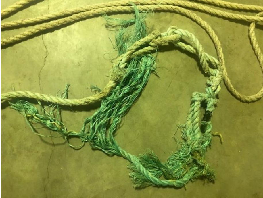
Fig. 5. Knotted section with two short sections of frayed 3/4-inch rope connected to float rope.
