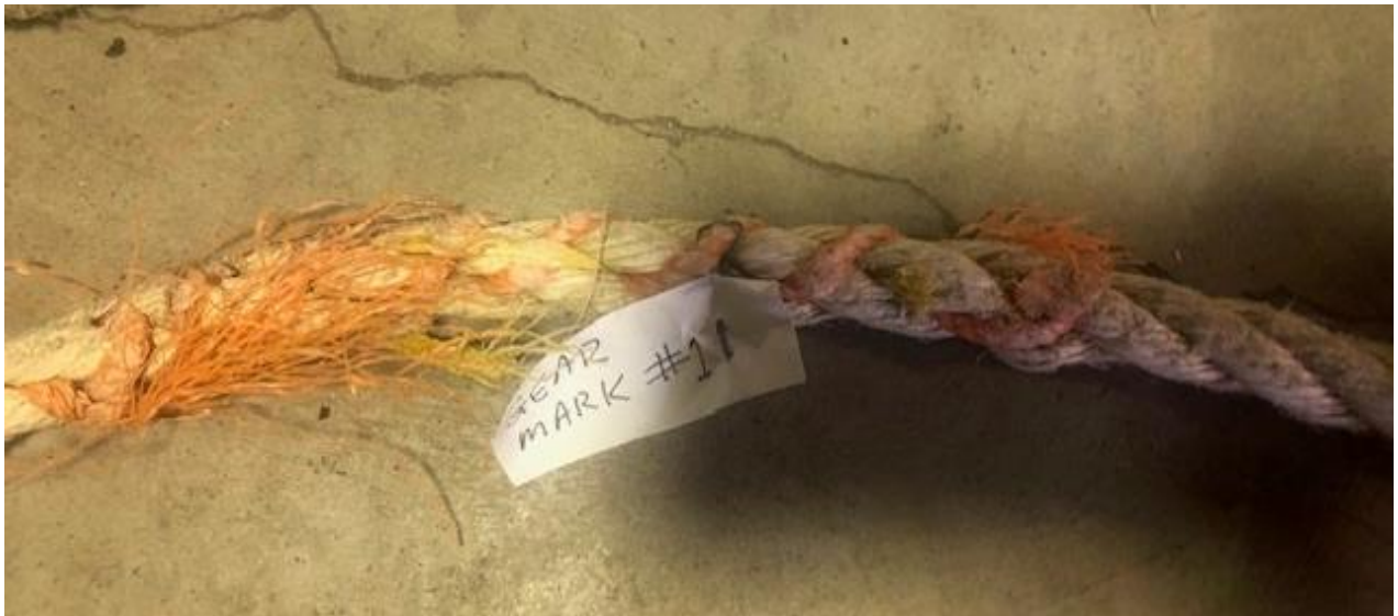
Fig. 6. First occurrence of orange and yellow twines interlaced on the same section of rope.
