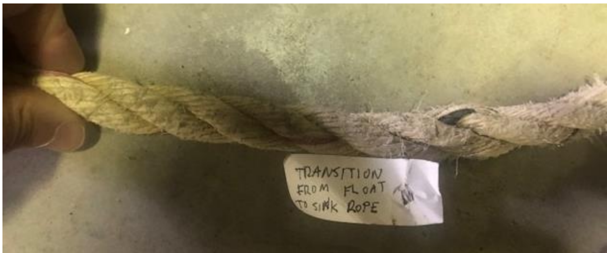
Fig. 4. Transition from float to sink rope, no occurrence of a splice.
