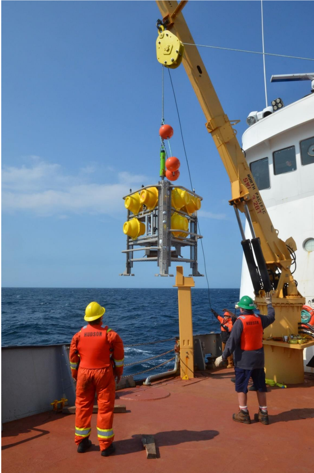
Figure 5.4. Lander deployment using acoustic release on winch rope and block on crane. The Lander is lowered to the ocean floor, then released acoustically with a transducer.
