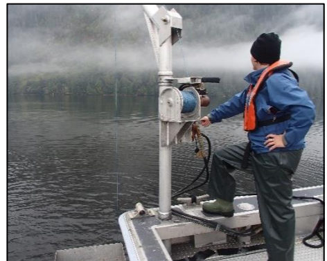
Image 1. Deploying a Van Veen Grab for benthic sampling.
