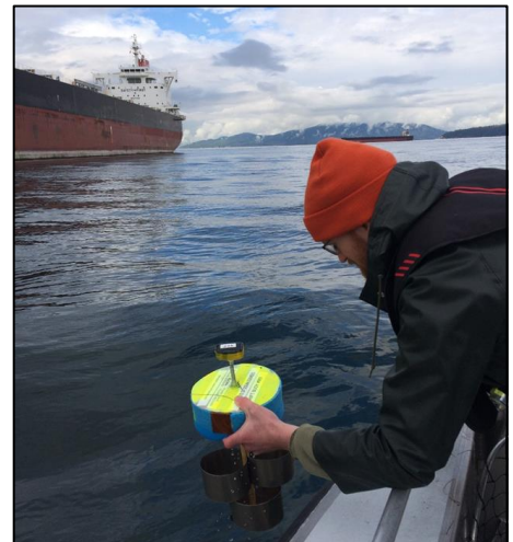
Image 1. Deployment of a current tracking drifter.
