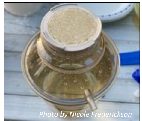
Image 2. Filtering sea water for biotoxin analysis.
