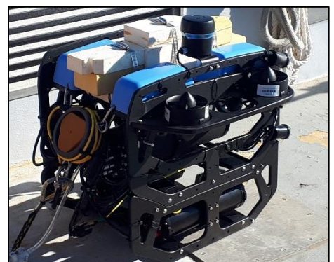
Image 1. "Blue ROV2" used to survey anchorage sites.
