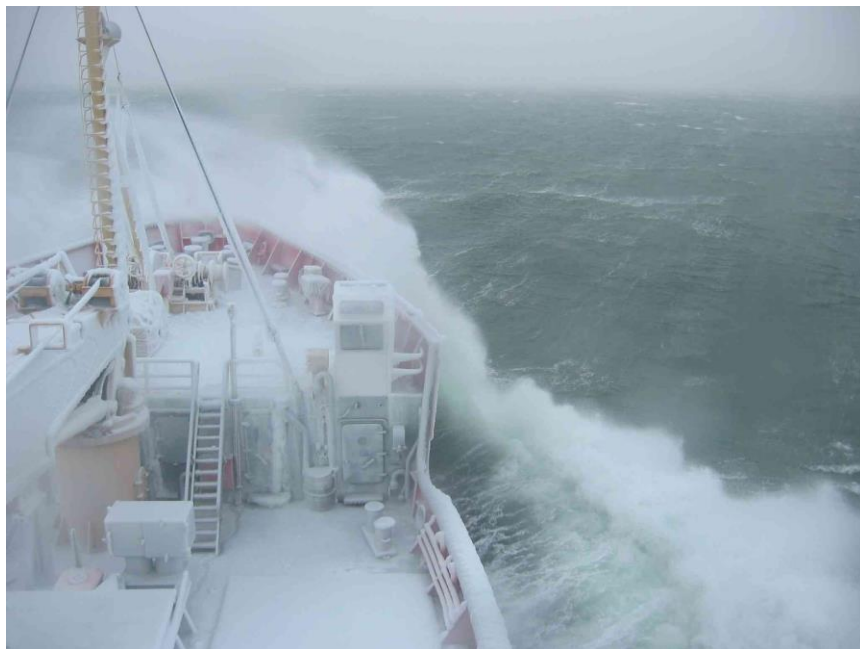
Figure 43 - Conditions de fort givrage (GCC)
