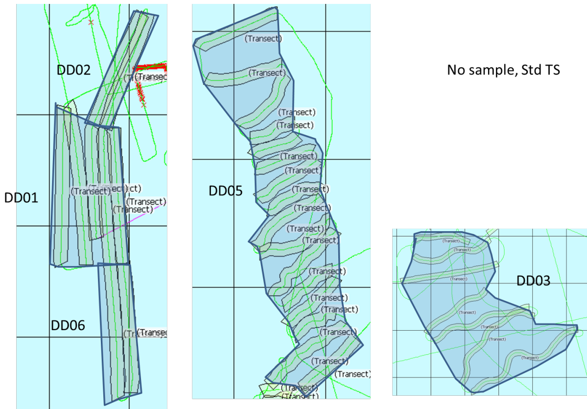
Figure 48. Trinity Ledge area Herring acoustic survey (#1) August 12, 2017, showing tracks conducted by the vessel Double Don . No samples were available. Standard Target Strength (TS) used.
