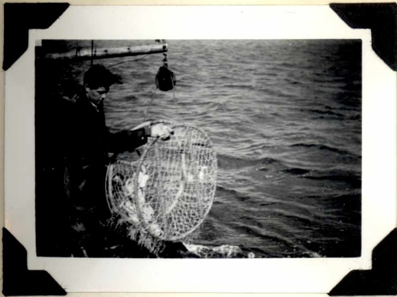
(4) Crab trap which has just been taken inboard. The boom, snatch block and trap line are shown. Note the crabs in the trap.
