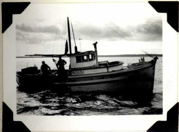
(3) Broadside view of crab fishing boat showing positions of fishermen and apparatus. The trap is ready to be taken inboard.
