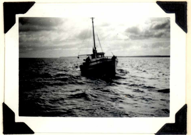
(2) Crab fishing boat on grounds, showing boom slung over side, the snatch block and the trap, which has just been pulled to the surface.
