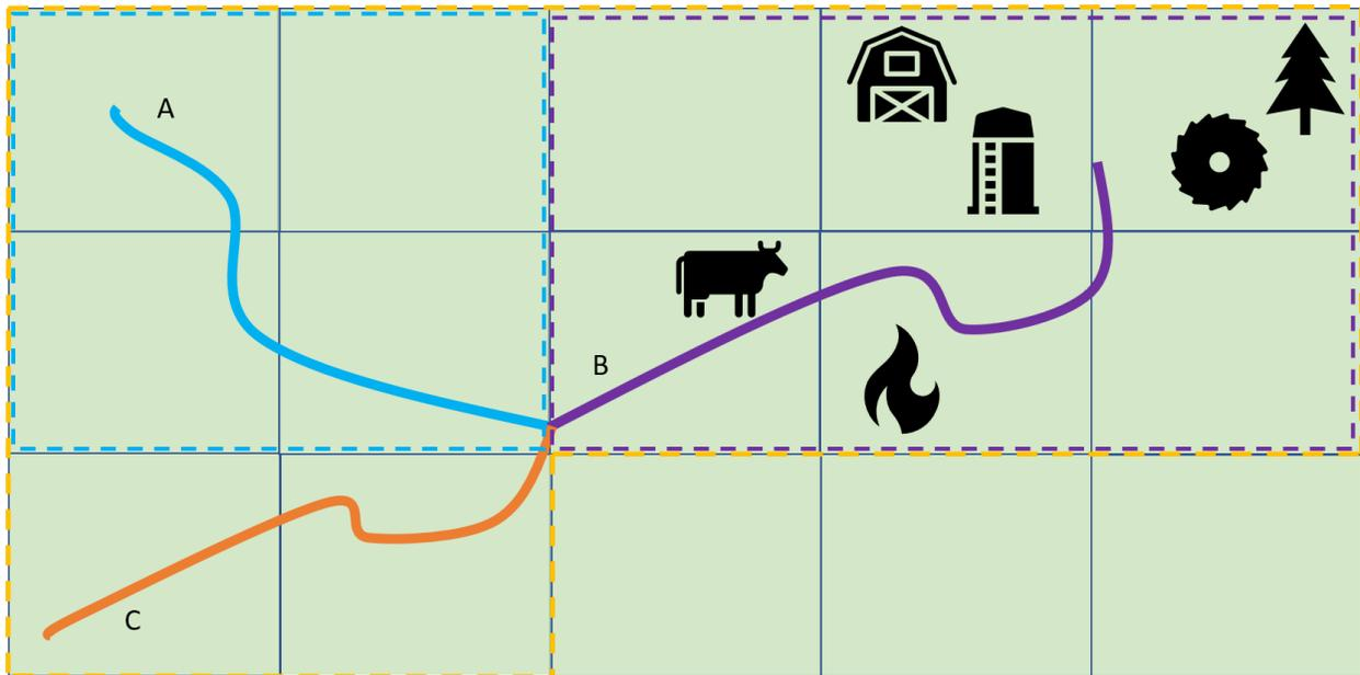
**Figure 3.** Stream reaches with associated catchment areas (dashed lines). Stream reach A would have a sedimentation threat score of 0, reach B would score 0.67, and reach C would score 0.33 (proportion of impacted cells per catchment area). The larger catchment area of reach C dilutes the landscape disturbance inputs from upstream.
