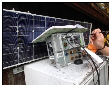
Image 2. Real time water temperature logger installation on Stuart River.
