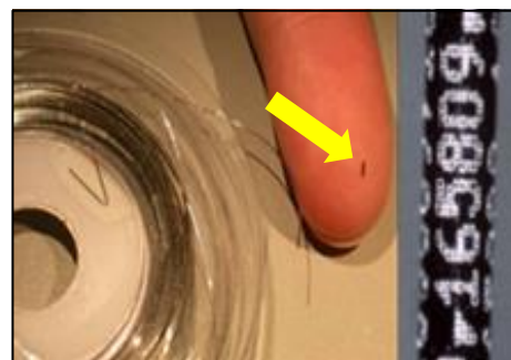
Image 2. Individual tags are cut from a spool of wire and are 1.1 mm long.
