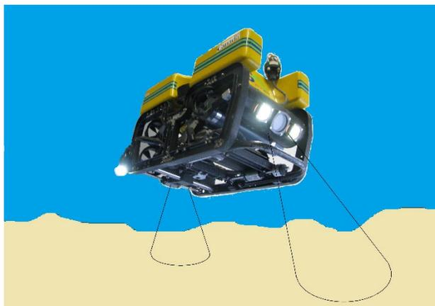
Figure 14: Diagram of a remotely operated vehicle (ROV) equipped with tandem forward-facing and downward-facing camera orientations for surveying the seabed (Sutherland et al. 2019a).
