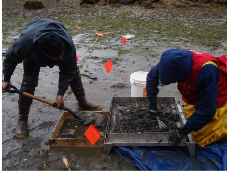
Figure 8: Sieving bivalve from sediment collected from a 0.25 m<sup>2</sup> sampling quadrat.
