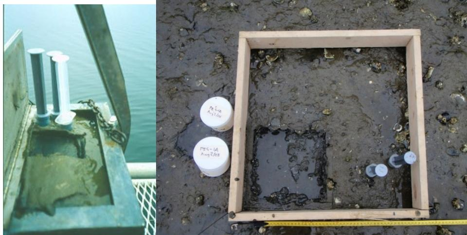
Figure 3: Syringe-cores deployed in a Ponar grab sample. A 2-cm deep surface scraping has been collected following syringe-core deployment. Note the black anoxic sediment underlying the oxic surface layer (~3 mm deep) (Left photo); Deployed syringe-cores and surface scraping within an intertidal sampling quadrat (0.25 m<sup>2</sup>) (Right photo).
