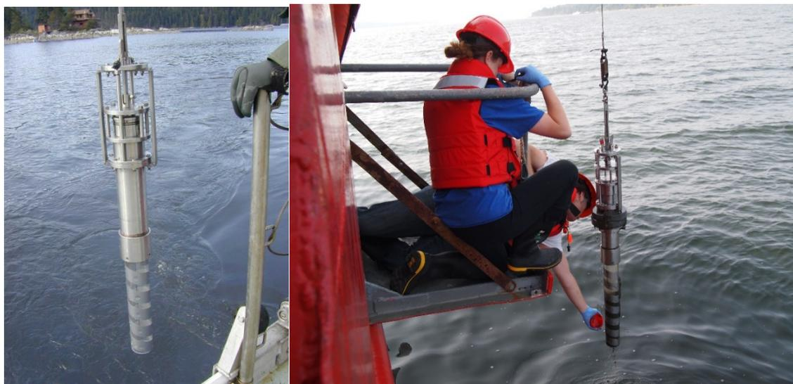
Figure 2: Gravity core (left photo); Retrieval of sediment core from gravity core deployment (right photo).
