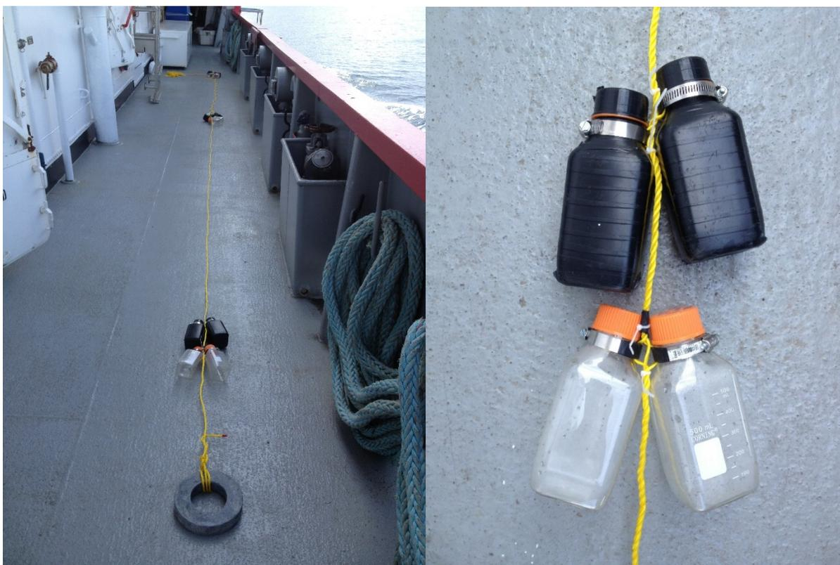
Figure 16: Primary productivity mooring showing 3 sets of duplicate light/dark incubation bottles at various water depths located above within, and below the chlorophyll-max layer (Left photo). A close up view of incubation bottles attached to mooring rope (Right photo).
