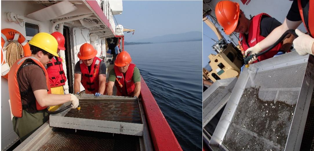
Figure 7: Sieving of a macrofauna grab sample using stacked sieves (1.0 cm, 0.5 mm) placed on a sieve table. In the right photo, the 1.0 cm sieve is in the background, while the macrofauna sample is being collected from the 0.5 mm sieve.
