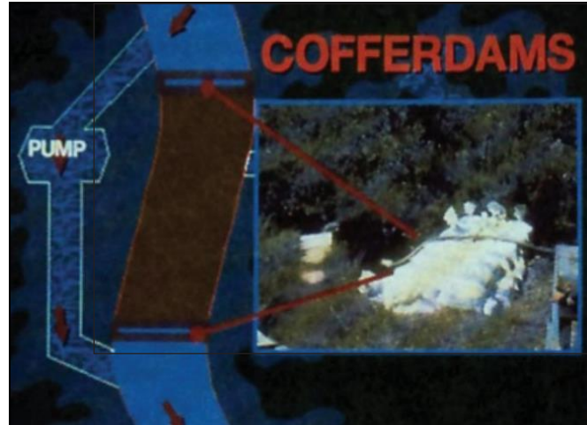
Figure 3.38 Cofferdams can be used in conjunction with temporary diversion channels to create a dry work area.
