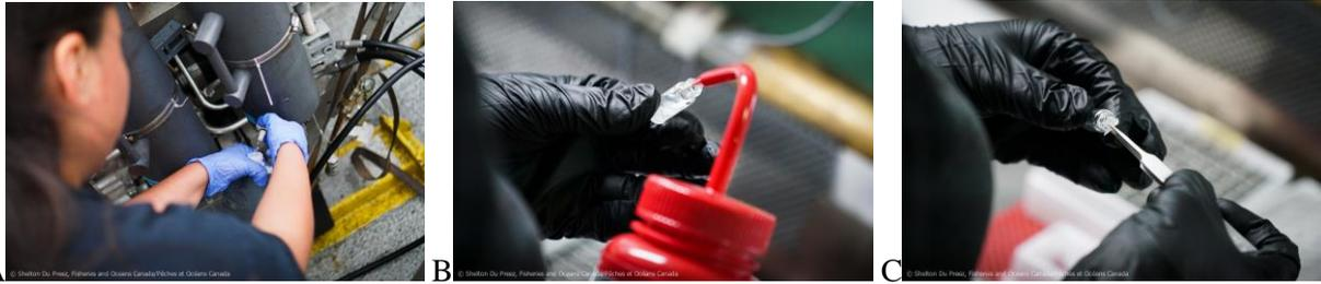
Figure 12. EDNA sampling procedure with A) Water extracted from the Niskin bottle (triggered to sample discrete sample of water at determine depth) B) DNA sample vials filled with 95% ethanol and C) Filters submerged in 95% ethanol for preservation (photo credits: Shelton Du Preez, DFO).
