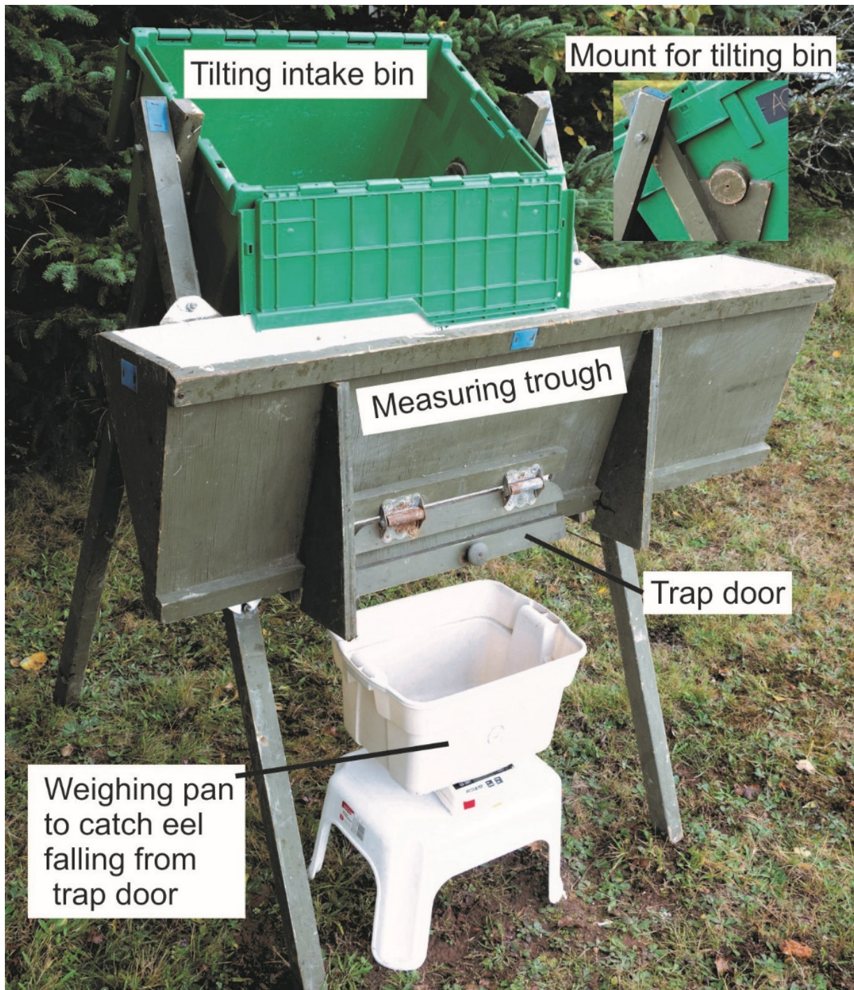
Fig. 15. A system for efficient eel measuring and weighing. An eel from the tilting intake bin is poured into the measuring trough, where its length is measured against an embedded metre stick. When the spring-loaded trap door is pulled open, the eel falls into the pan where it is weighed. The legs are detachable from the trough for transport and storage. The inset shows how the intake bin is mounted on brackets that are attached to the legs.
