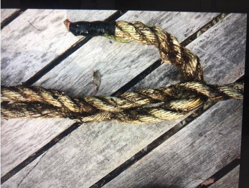
Exhibit B: Two tucks between strands of 5/8 inch diameter float rope adjacent to the 19 inch loop removed from Cottontail on October 19, 2020.
