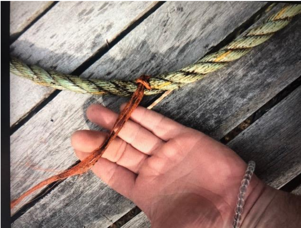
Exhibit C: Orange braided twine (length 8 inches) tucked once through 5/8 inch diameter float rope at a distance of approximately 8 fathoms from the 19 inch loop removed from Cottontail on October 19, 2020.
