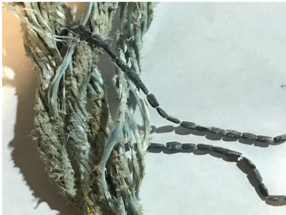
Exhibit E: Beaded lead filaments exposed from a segment of the sinking rope removed from Cottontail on March 10, 2021.
