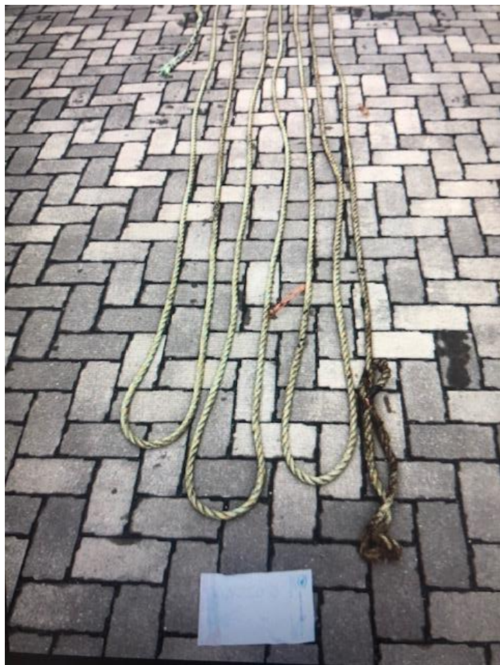
Exhibit A: Approximately 97 ft of 5/8 inch diameter float rope, including a 19 inch loop, that was removed from Cottontail on October 19, 2020 and laid out on the ground.
