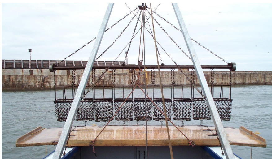
Figure 2. Nine bucket Digby-type dredge commonly used to fish sea scallops in the Gulf Region.
