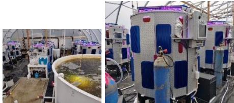
Top and side view of installed photobioreactor used for phytoplankton production.
