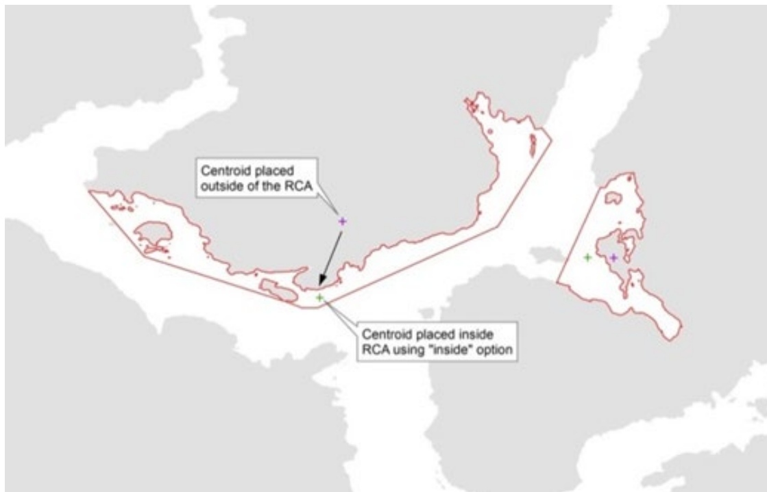
Figure 3. An example of an RCA (Walken Island to Hemming Bay) where the centroid determined to be outside the RCA was 'forced' inside the RCA.
