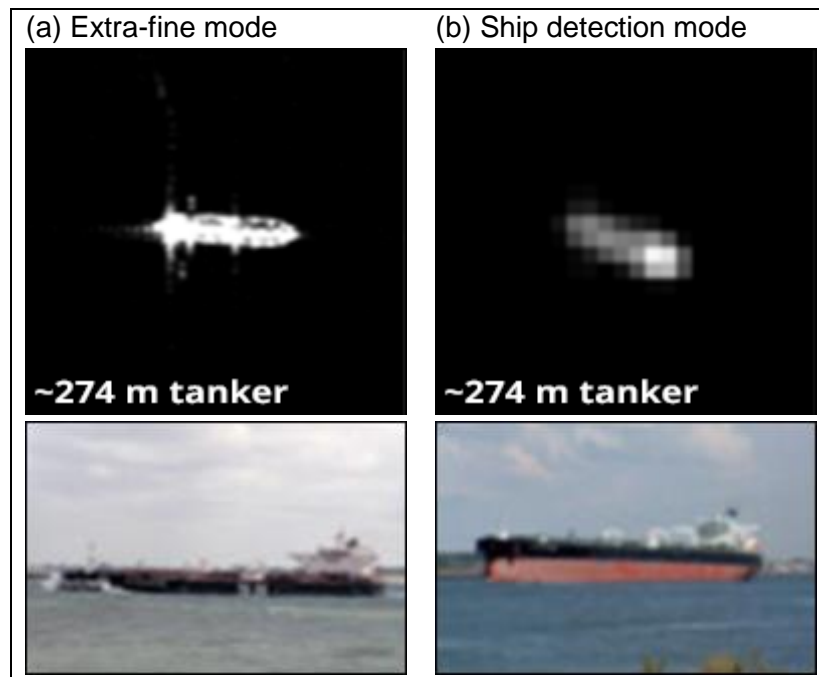
Figure 7. Synthetic Aperture Radar images from RadarSat II (top panel) using (a) 'extra-fine' and (b) 'ship detection' (DVWF) beam modes. Pictures are from MDA ( https://mdacorporation.com/geospatial/international/markets/defence-and-security ).
